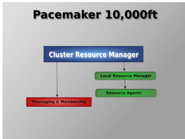
Figure 1.4. Conceptual overview of the cluster stack
